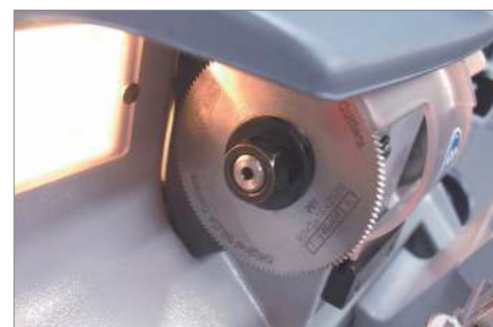
Prismatic cutter made of HSS
